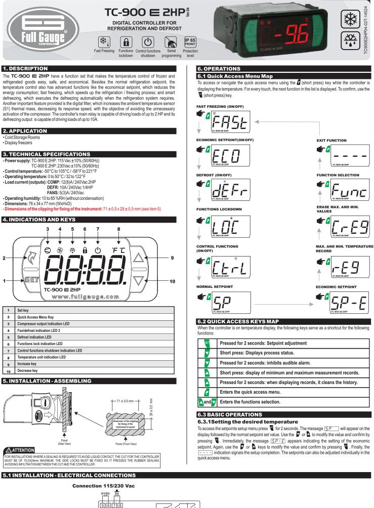
\*The sensor S1 (black) must be in the ambient. \*The sensor S2 (gray) must be placed in the evaporator through metallic cramp. EVOLUTION
